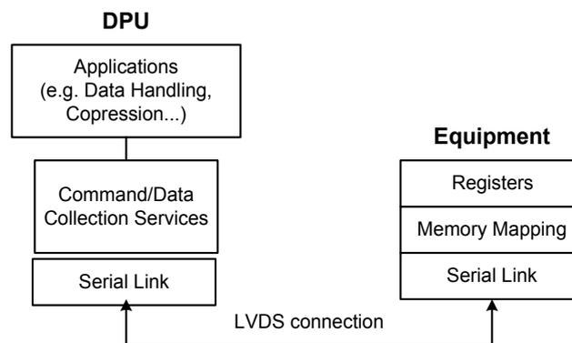
Figure 19 Communication Stack.
