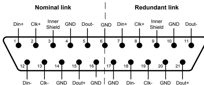
Figure 17 View of the Serial Link front plug on equipment side.
