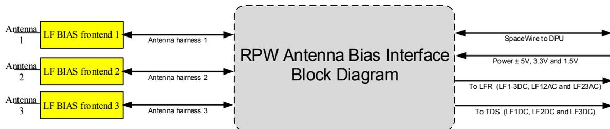
Figure 13 BIAS unit interface diagram.
