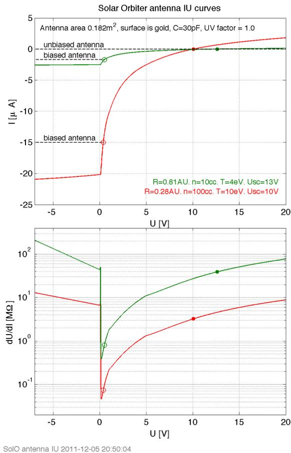
Figure 1 Expected antenna IU curves and resistance.
