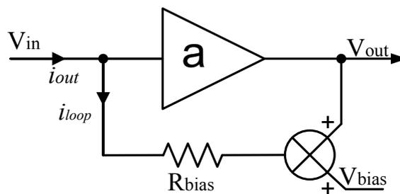
Figure 15 Principle of positive feedback for creating a constant current source.
