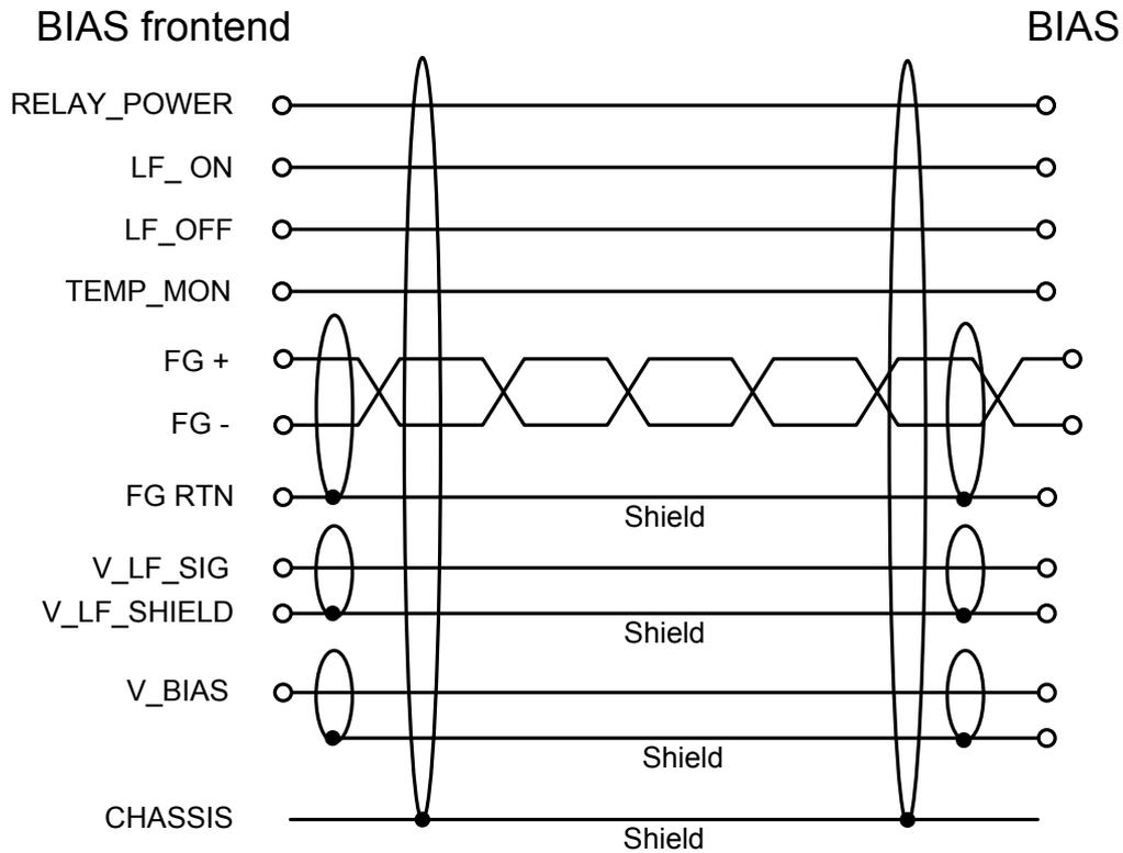
Figure 16 LF BIAS frontend harness configuration.
