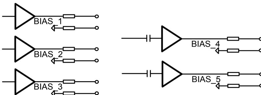
Figure 14 BIAS unit analogue signal interfaces. LFR takes all five outputs, whereas TDS takes outputs BIAS\_1, BIAS\_2 and BIAS\_3 (DC only).
