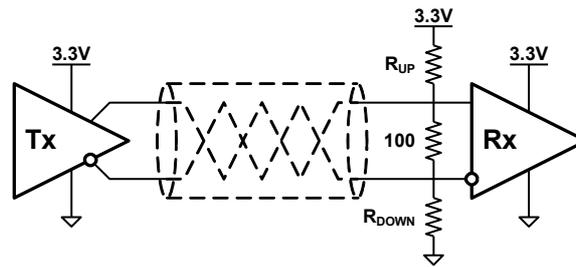
Figure 18 Over-voltage protection.
