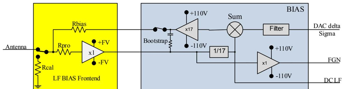
Figure 6 Floating Ground Concept.
