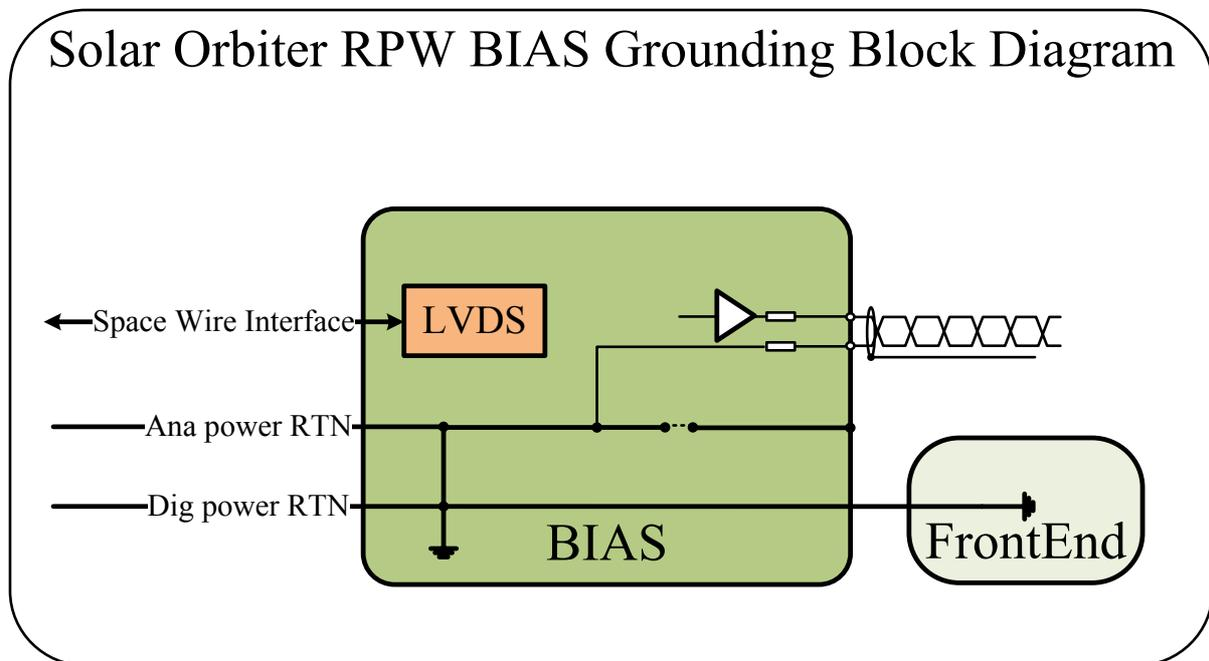
Figure 12 BIAS grounding block diagram diagram.
