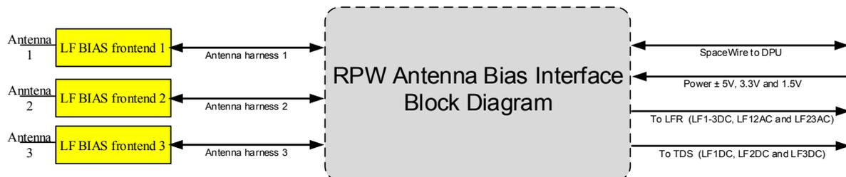
Figure 13 illustrates both the internal and external BIAS sensor interfaces, with outputs to LFR and TDS. BIAS is connected to each antenna through the LF BIAS frontends, located in the RPW preamplifier boxes.
