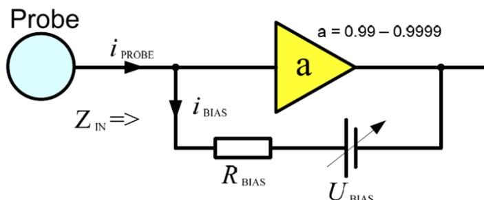
Figure 5 Principle of ANT Current Biasing.
